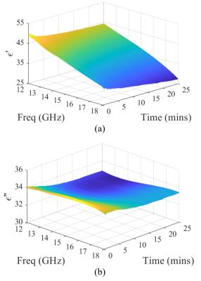
Figure 5. Sediment monitoring of 2 mg/ml yeast cell suspension for 25 minutes: (a) real part, (b) imaginary part.
