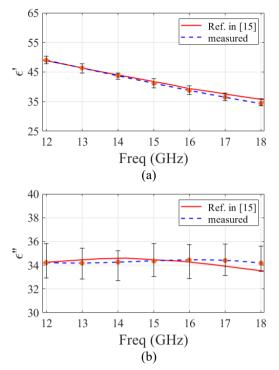
Figure 4. Extracted permittivity of 2 mg/ml yeast cell suspension: (a) real part, (b) imaginary part.
