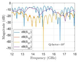
Figure 3. S-parameters of the system with  $S_{21}$  (15 GHz) tuned below -70 dB, Q-factor =  $10^4$ .
